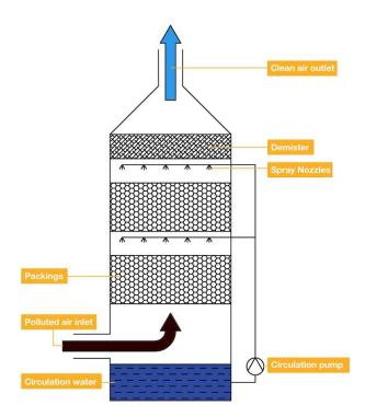
The scrubbed gas then undergoes a separation process to remove any remaining water droplets and is discharged through the outlet. The water containing the captured pollutants is carefully treated or disposed of according to environmental regulations.
